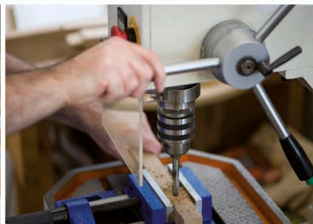
4 When you have aligned the workpiece, start the machine and turn the wheel to lower the drill onto the wood. Drilling will stop automatically when the desired depth is reached.
