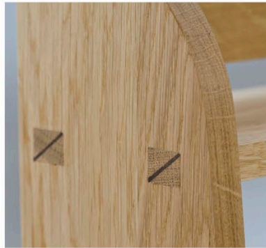
WEDGED TENON DETAIL
