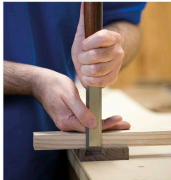
PARING VERTICALLY WITH A GUIDE
