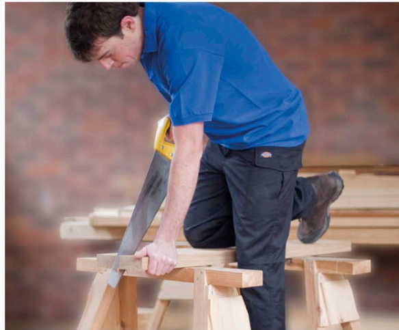
RIPPING ON TRESTLES
