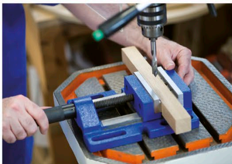
3 To hold the workpiece securely, use drill vises, which can be fixed to the drill table and allow safe working. Alternatively, use C-clamps or jigs to hold and position the work.
