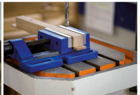
5 If the holes will be visible on the face of the workpiece, place a cutoff piece underneath as you drill. This will prevent any breakout on the surface of the wood as the drill emerges.
