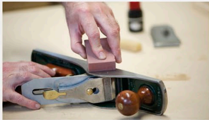
CLEANING WITH AN ABRASIVE BLOCK
