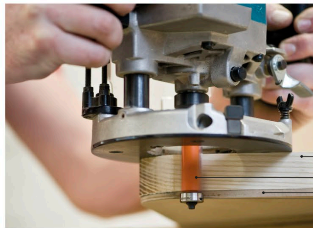
CUTTING A PROFILE WITH A BEARING-GUIDED CUTTER
