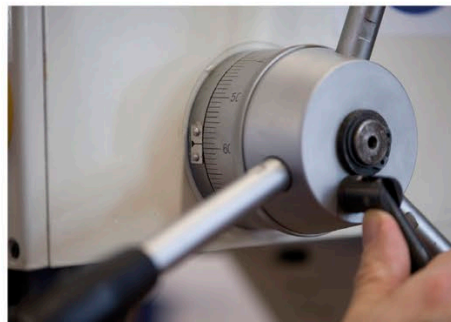
1 To set the depth , lower the drill to the required depth by rotating the depth gauge and stop wheel on the side of the machine. Use the scale on top of the wheel to fix the depth.
