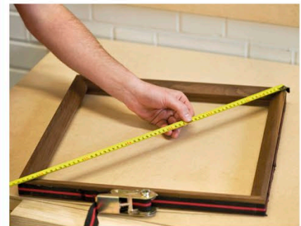
CHECKING SECOND DIAGONAL
