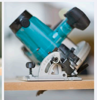
CUTTING AT AN ANGLE
