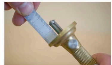
USING A TAPE MEASURE TO SET A GAUGE
